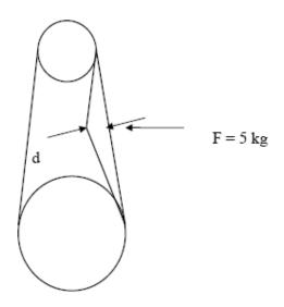
The belt should not move by more than 2 mm if a pressure of 5 kg is applied.
